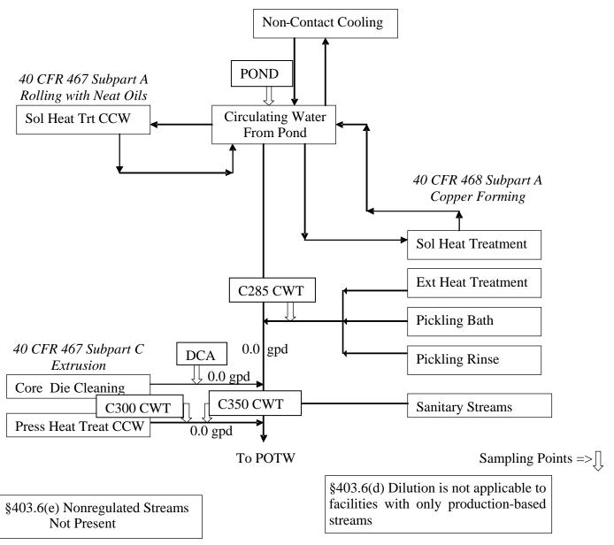
If a stream is not present, show NOT PRESENT or N/P. If a stream is present, the wastewater can enter the POTW but currently has no flow, show 0.0 gpd. If a stream is present but the wastewater cannot enter the POTW, show Zero Discharge or Z/D. If an unregulated stream is present but the User has decided not to declare it at this time, show N/P.
